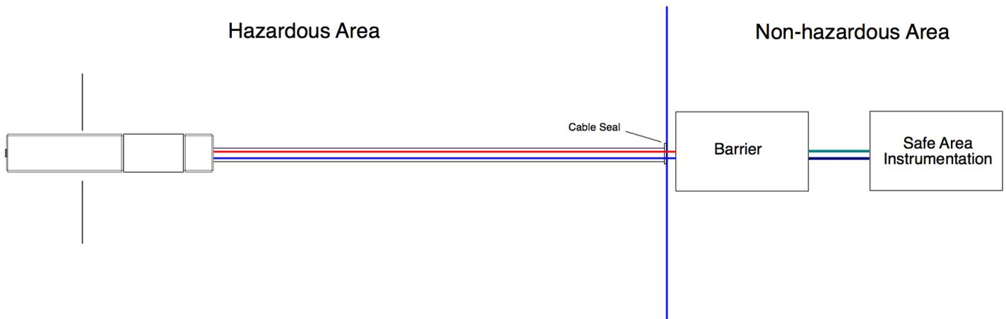
Figure 1: Typical connection arrangements
