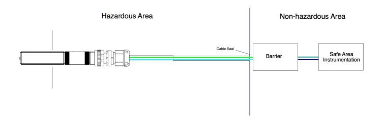
Figure 1: Typical connection arrangements
