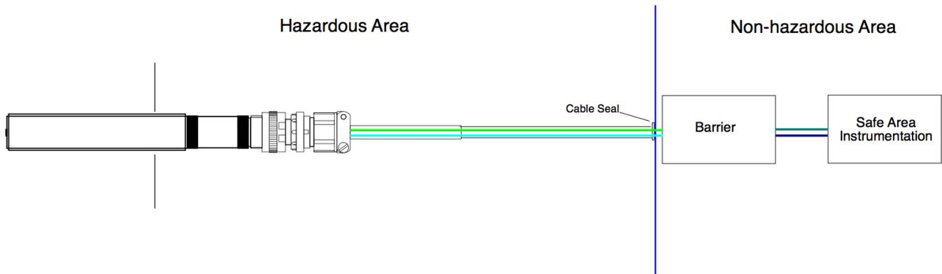
Figure 1: Typical connection arrangements
