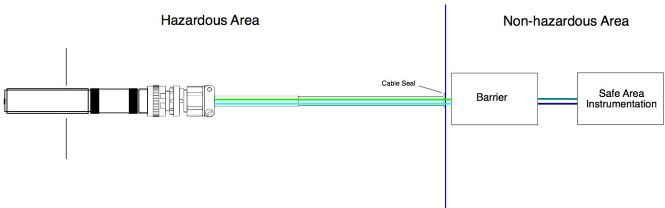
Figure 1: Typical connection arrangements
