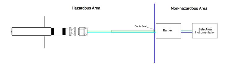
Figure 1: Typical connection arrangements
