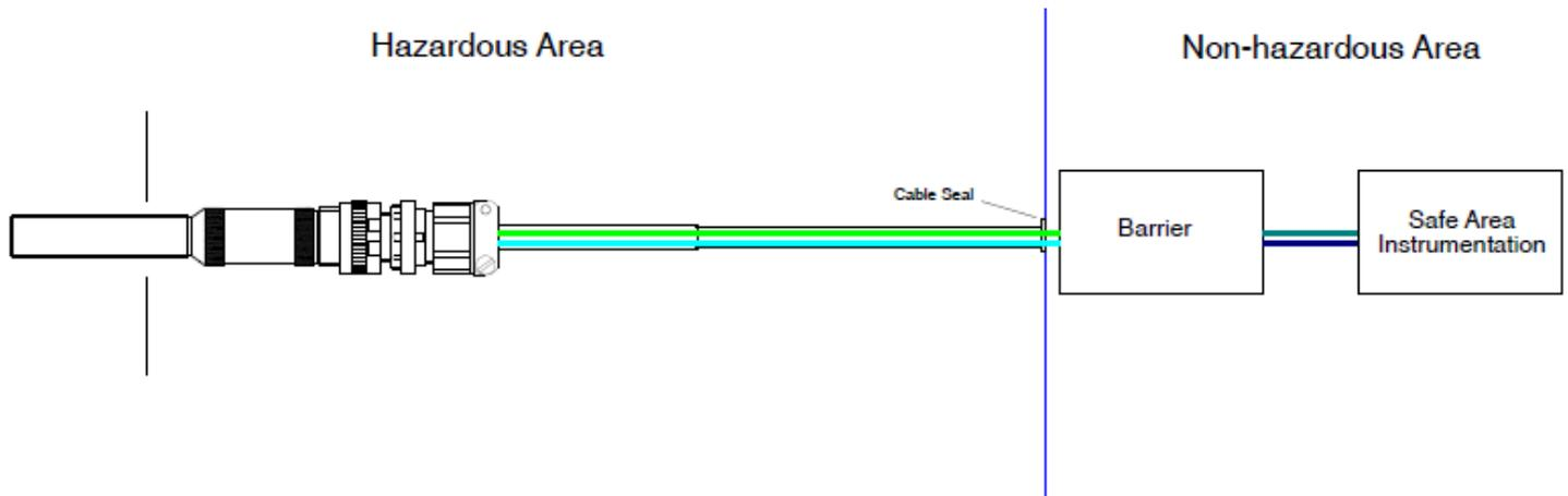
Figure 1: Typical connection arrangements
