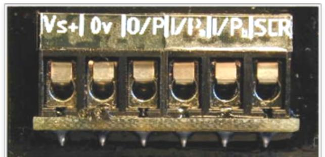
2. Preferably the input signal to the module should be via twin-core screened cable and the output from the module should also be via twin-core screened cable.
