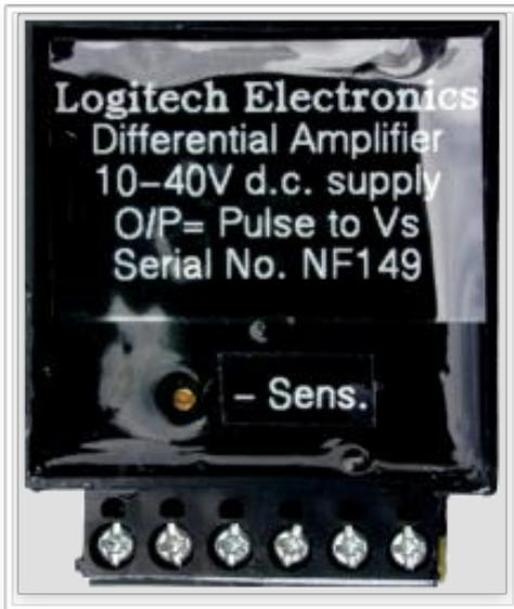
Differential Amplifier Module type **DIFF1** is a self-contained signal conditioning module designed to be used with any of the **Logitech Electronics** range of standard Magnetic Pick-ups.
