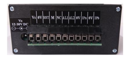
The image above shows the rear panel of a standard 2000T MKIII instrument. The actual terminals available on the rear panel will vary depending on the model. Below are the definitions of each of the terminals that may be present. Refer to the terminal labels on the instrument and match these with the functions below.
